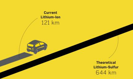
If the barriers to commercialization can be overcome, lithiumsulfur batteries could carry electric vehicles roughly five times further than today's standard lithiumion hatteries
