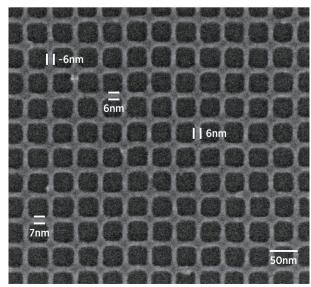
Light-emitting ZnS nanostructures can be patterned into nearly any shape, including grids as above, using a multipurpose photoresist.
