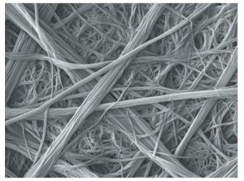
This scanning electron microscope image shows that the artificial ion channels self-assemble into fibers.
