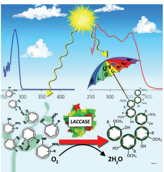
A lignin-like short chain oligomer (right) absorbs UV light far more effectively than its component monomers (left).
