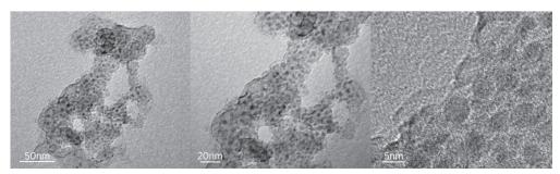
Transmission electron microscopy images of (left, center) nickel-silica catalyst and (right) a commercial catalyst.
